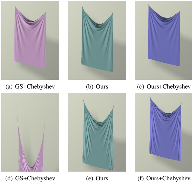
Figure 11: Tablecloth examples simulated by Projective Dynamics using a large time step \Delta t = 1/30s and the same real-time budgets. Cloth in the first row have 10k vertices. Cloth in the second row have 40k vertices.
